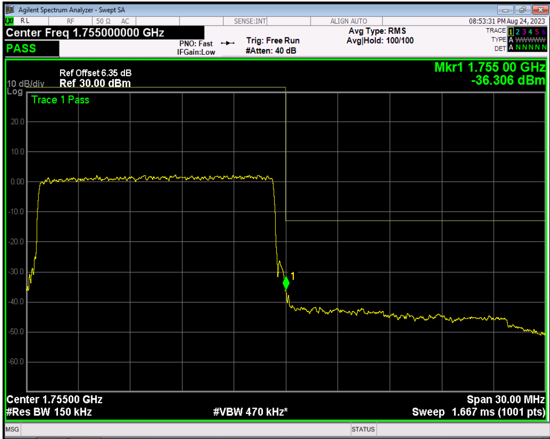
Band4 16QAM BW=15MHz Channel=20325 RB Size=75 Position=#0
