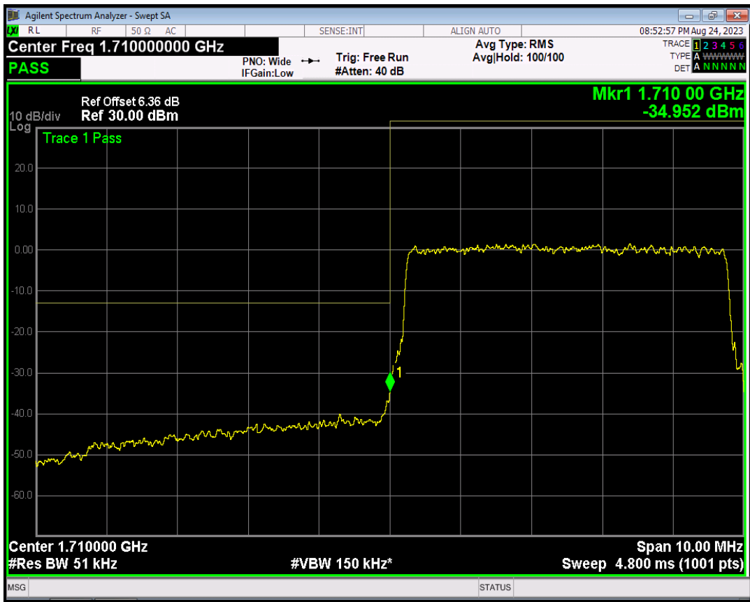
Band4 QPSK BW=5MHz Channel=20375 RB Size=25 Position=#0
