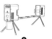
5. The external machine is placed outdoors and the internal machine is placed indoors
