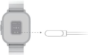
Align the charging cable with the top pin on the bottom case boss until the charging indicator appears on the watch screen.
