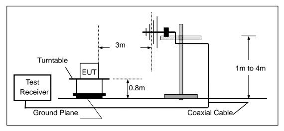
(c) For radiated emissions above 1000MHz
