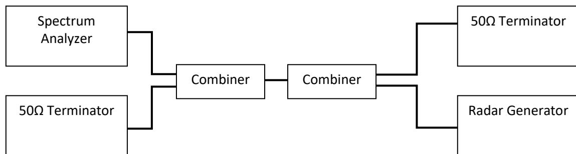
**TEST REPORT****3.8 Radar Waveform Calibration Procedure**
