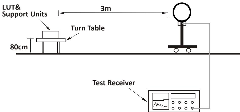
For Radiated emission 30MHz to 1GHz:
