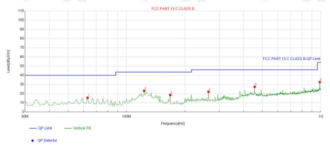
Suspected List Freq. Factor Limit Margin Reading Level Height Angle NO. Polarity [MHz] [dB]  $[dB\mu V/m]$  $[dB\mu V/m]$  $[dB\mu V/m]$ [dB] [cm] [°] 63.013013 -14.38 29.91 15.53 40.00 24.47 100 108 Vertical 123.21321 -15.99 39.10 43.50 20.39 Vertical 2 23.11 100 19 167.87787 -16.99 35.60 18.61 43.50 24.89 100 Vertical 138 264.00400 4 -12.71 34.79 22.08 46.00 23.92 100 168 Vertical 456.25625 5 -8.37 35.85 27.48 46.00 18.52 100 1 Vertical 6 987.37737 0.38 32.26 32.64 54.00 21.36 100 168 Vertical
