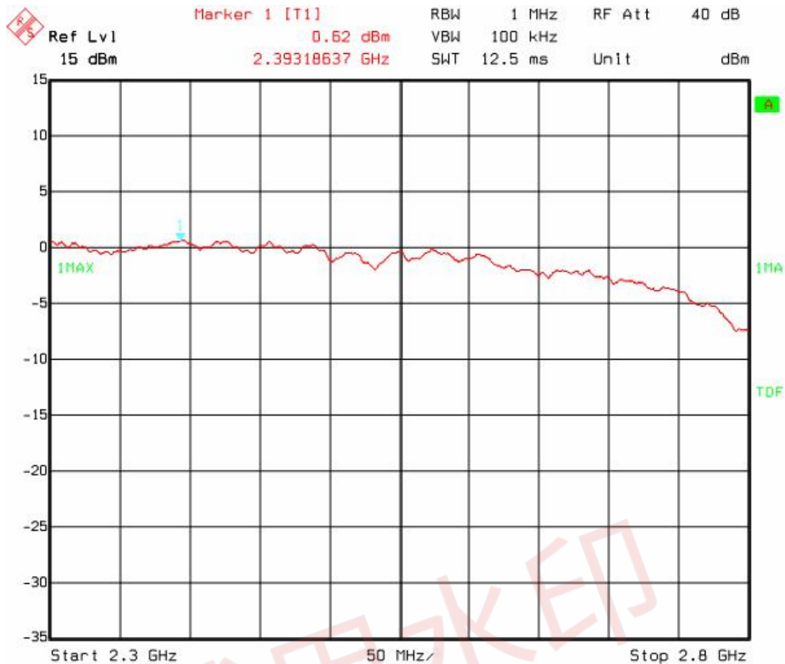
Figure 16: Output Power, USB Dongle in Laptop
