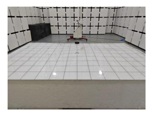
Set-up for Radiated Spurious Emission, Above 1GHz
