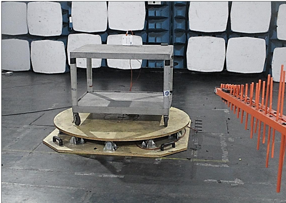
Figure 40 - Test Setup - 30 MHz to 1 GHz - Z Orientation
