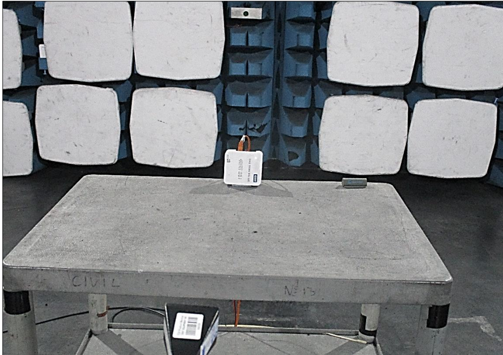
Figure 42 - Test Setup - 18 GHz to 30 GHz - Z Orientation
