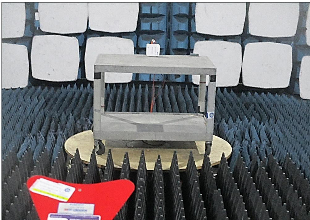
Figure 40 - Test Setup - 30 MHz to 1 GHz - Z Orientation
