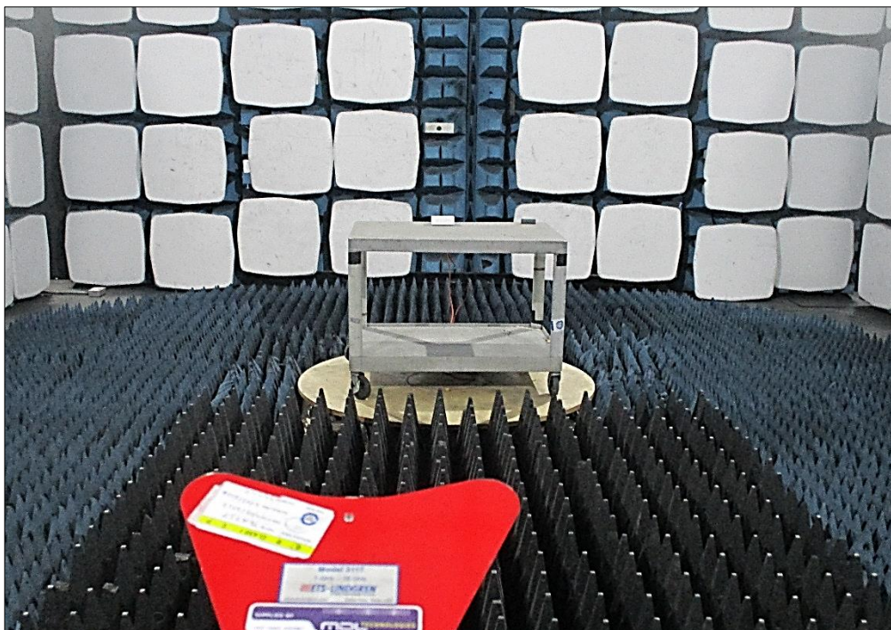
Figure 34 - Test Setup - 30 MHz to 1 GHz - X Orientation
