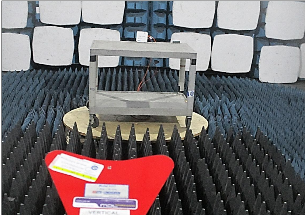
Figure 38 - Test Setup - 1 GHz to 18 GHz - Y Orientation
