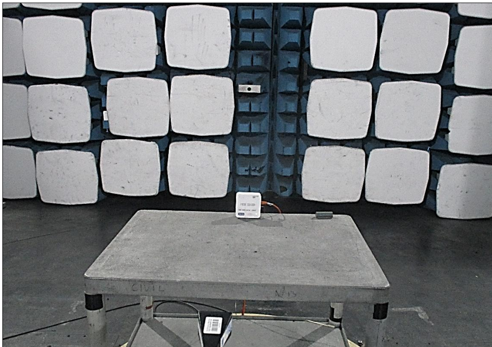
Figure 38 - Test Setup - 1 GHz to 18 GHz - Y Orientation
