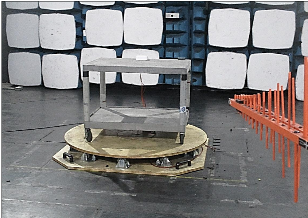
Figure 34 - Test Setup - 30 MHz to 1 GHz - X Orientation
