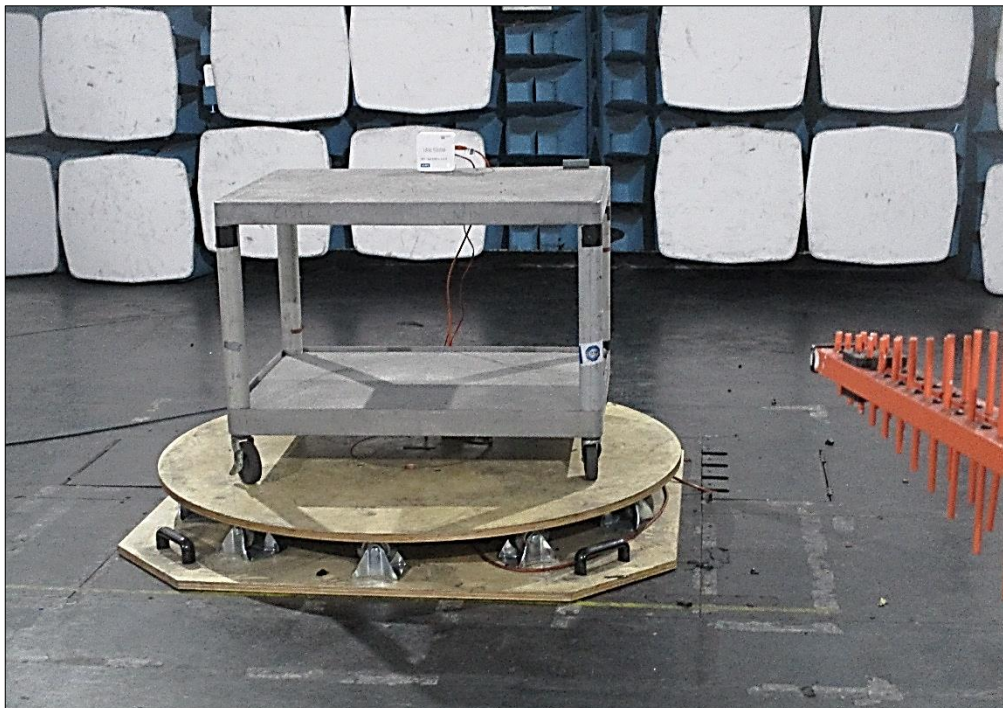
Figure 36 - Test Setup - 18 GHz to 30 GHz - X Orientation
