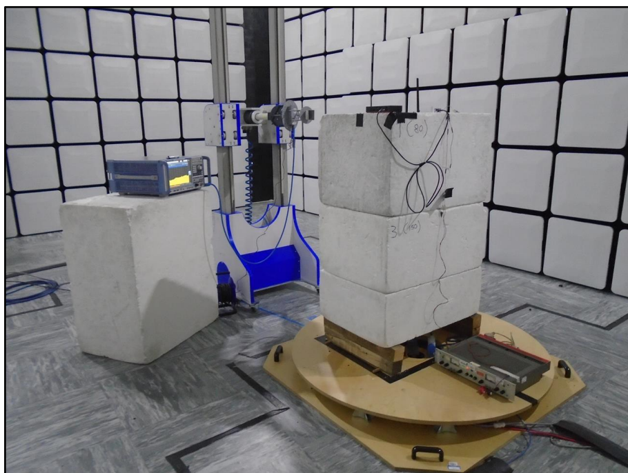
Figure 20 - Test setup, External Antenna - 18 GHz to 30 GHz
