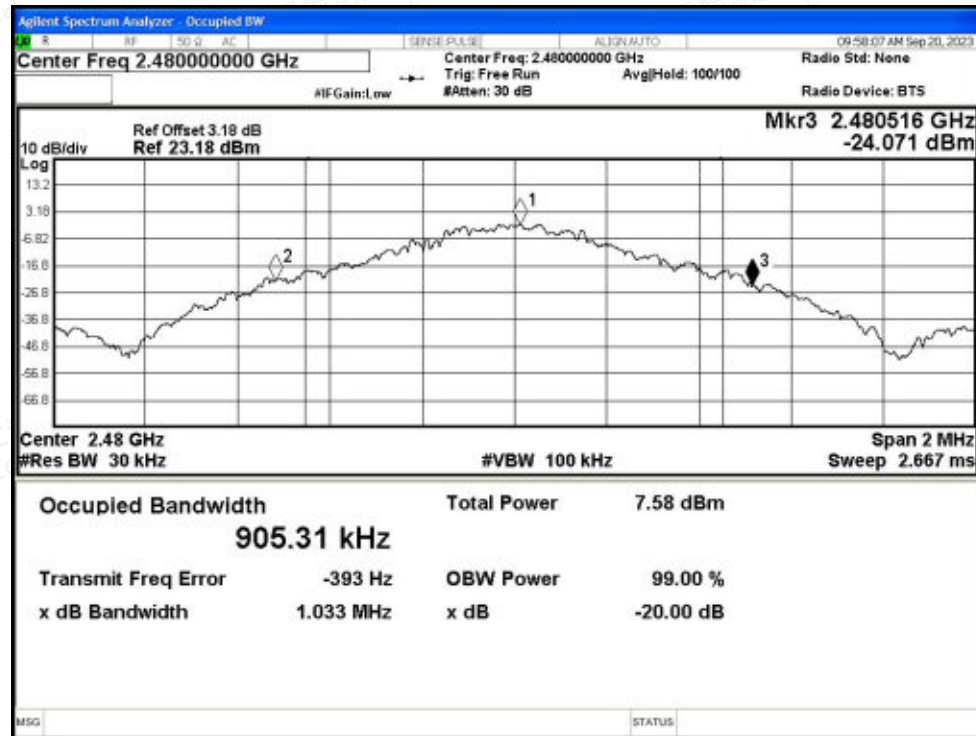
-20dB Bandwidth NVNT 2-DH5 2402MHz Ant1
