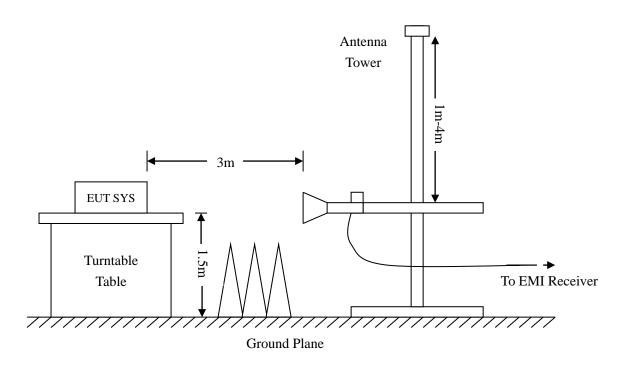
Frequency:9kHz-30MHz Frequency:30MHz-1GHz Frequency: Above 1GHz RBW=10KHz, RBW=120KHz, RBW=1MHz, VBW=300KHz VBW = 30KHzVBW=3MHz(Peak), 10Hz(AV) Sweep time= Auto Sweep time= Auto Sweep time= Auto Trace = max hold $Trace = max \ hold$ Trace = max holdDetector function = peak Detector function = peak, QP Detector function = peak, AV
