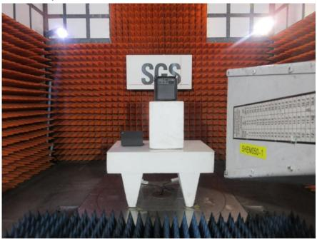
Conducted Emissions at AC Power Line (150kHz-30MHz)
