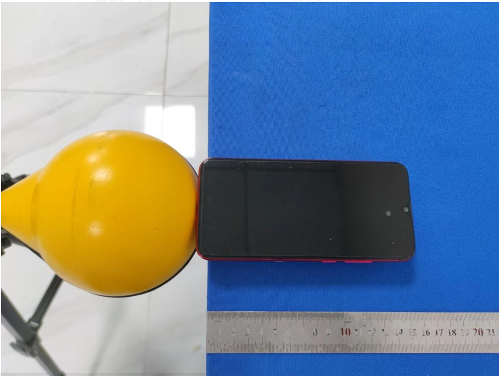
Test Position C(0cm) - Exposure photo from side edge surface-Left(TM1)
