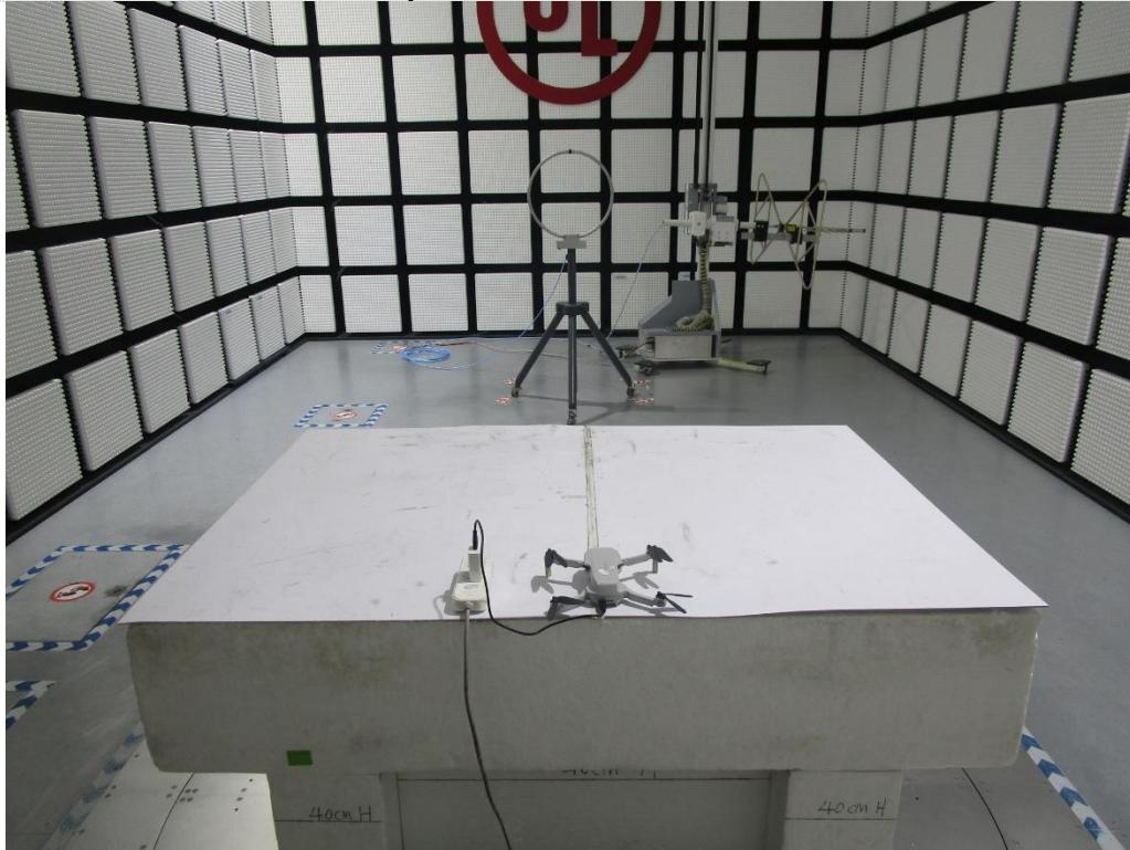
**Radiated Spurious Emission Below 1 GHz and 30 MHz**
