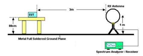
For radiated emissions from 30MHz to 1GHz
