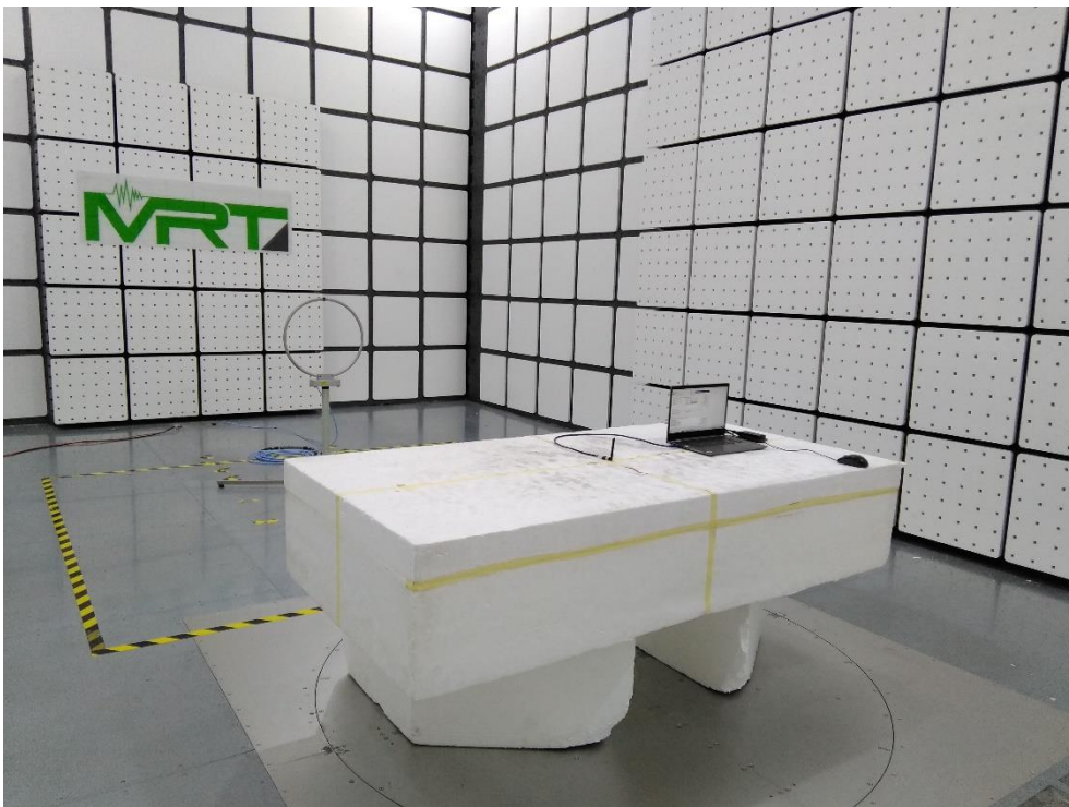
Description: Radiated Emission Test Setup for 9kHz~30MHz
