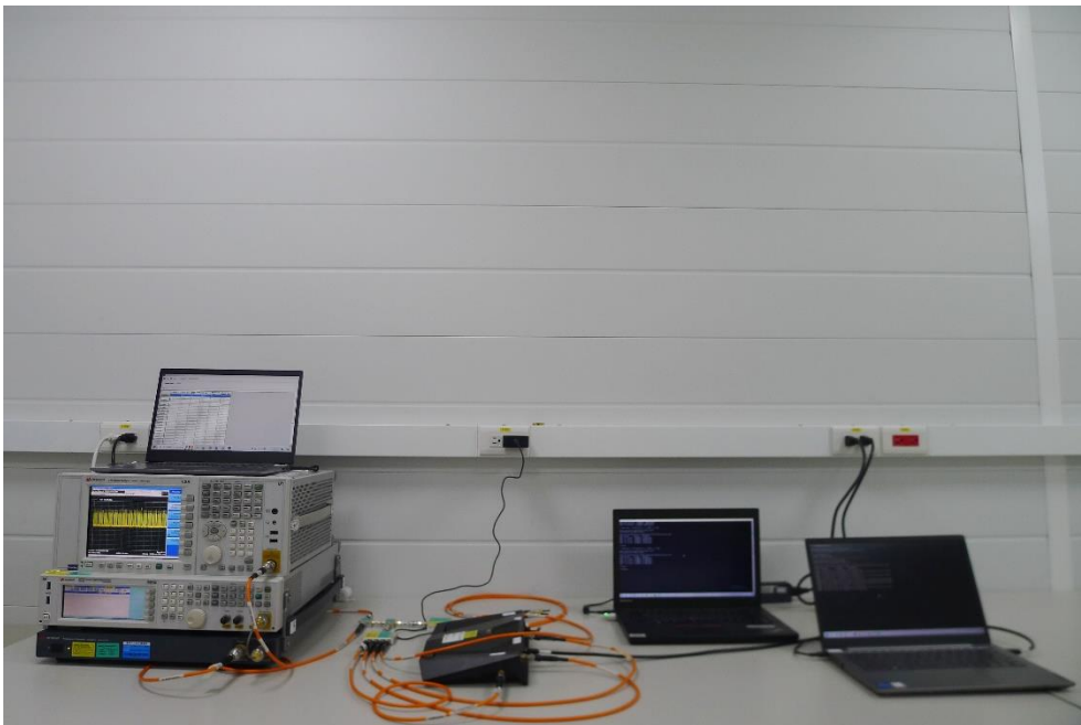
Description: DFS Test Setup
