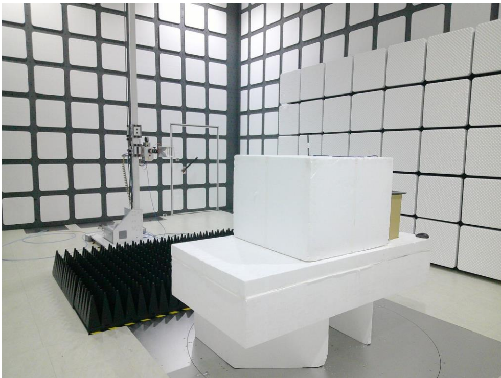
Description: Radiated Emission Test Setup for 1GHz~18GHz
