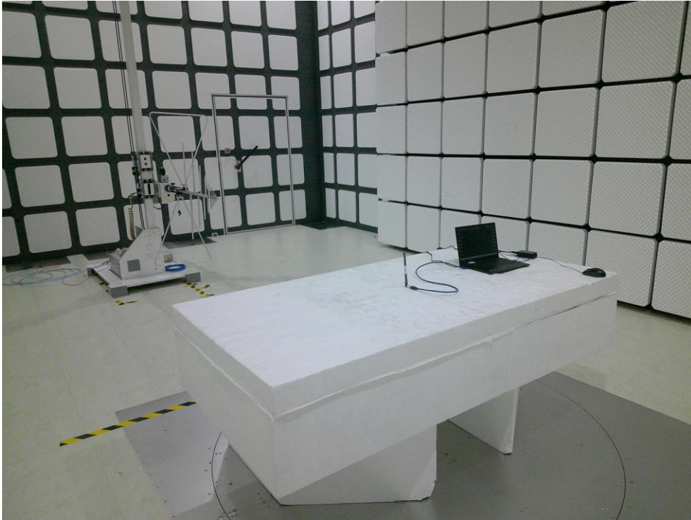
Description: Radiated Emission Test Setup for 1GHz~18GHz
