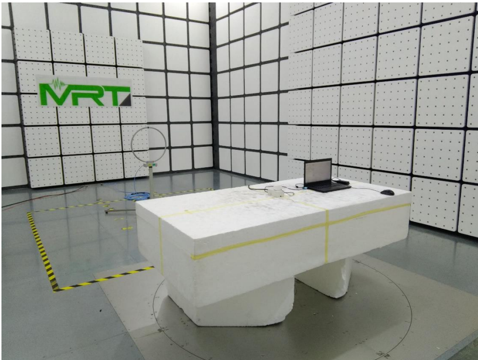
Description: Radiated Emission Test Setup for 9kHz~30MHz
