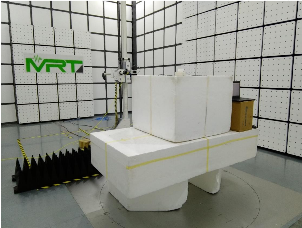
Description: Radiated Emission Test Setup for 9kHz~30MHz
