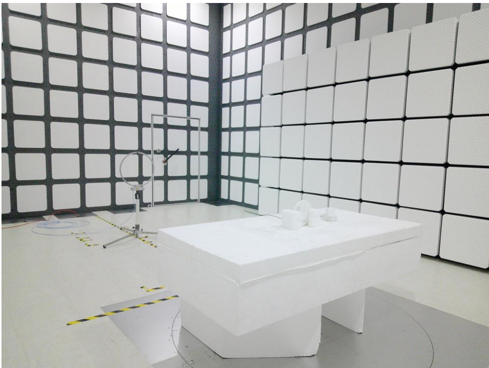
Description: Radiated Emission Test Setup for 9kHz~30MHz
