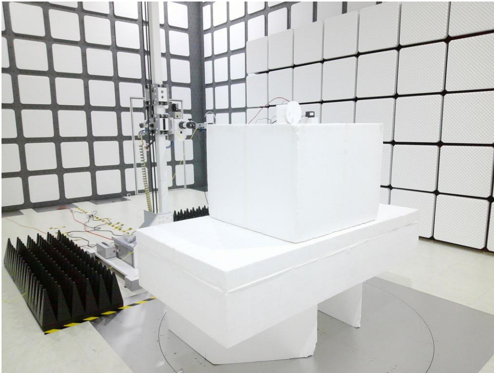
Description: Radiated Emission Test Setup for 9kHz~30MHz
