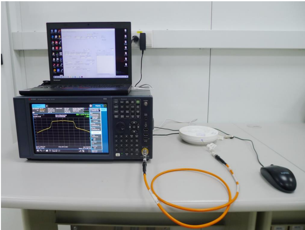
Description: Conducted Emission Test Setup - BLE
