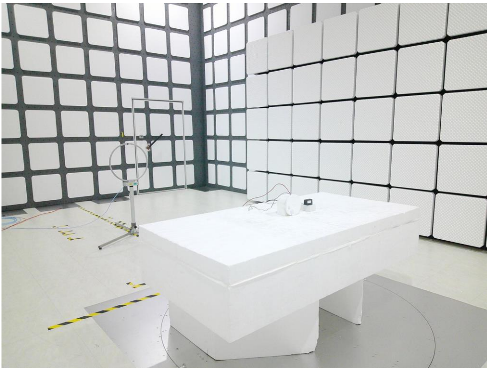
Description: Radiated Emission Test Setup for 9kHz~30MHz
