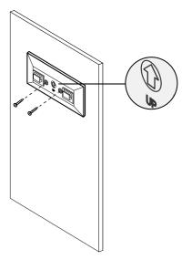
2. Attach the EAP to the base as shown in the figure.
