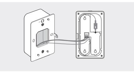
5. Attach the EAP to the mounting bracket. Secure them with the provided screw.
