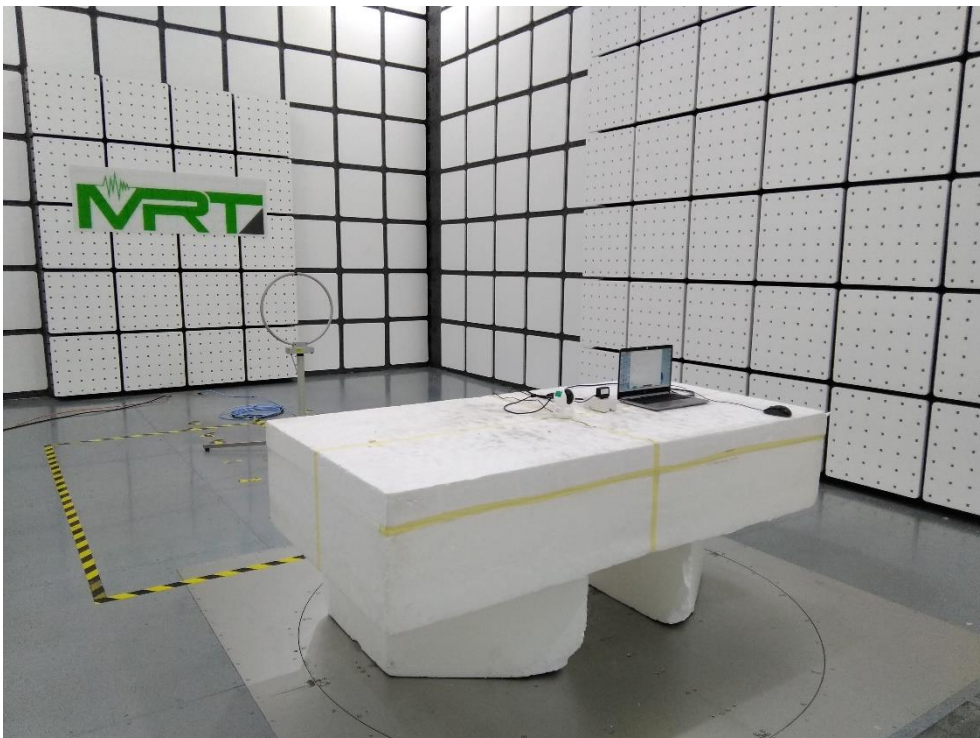
Description: Radiated Emission Test Setup for 9kHz~30MHz
