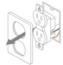
**3 Identify** the wires and disconnect the old wires.
