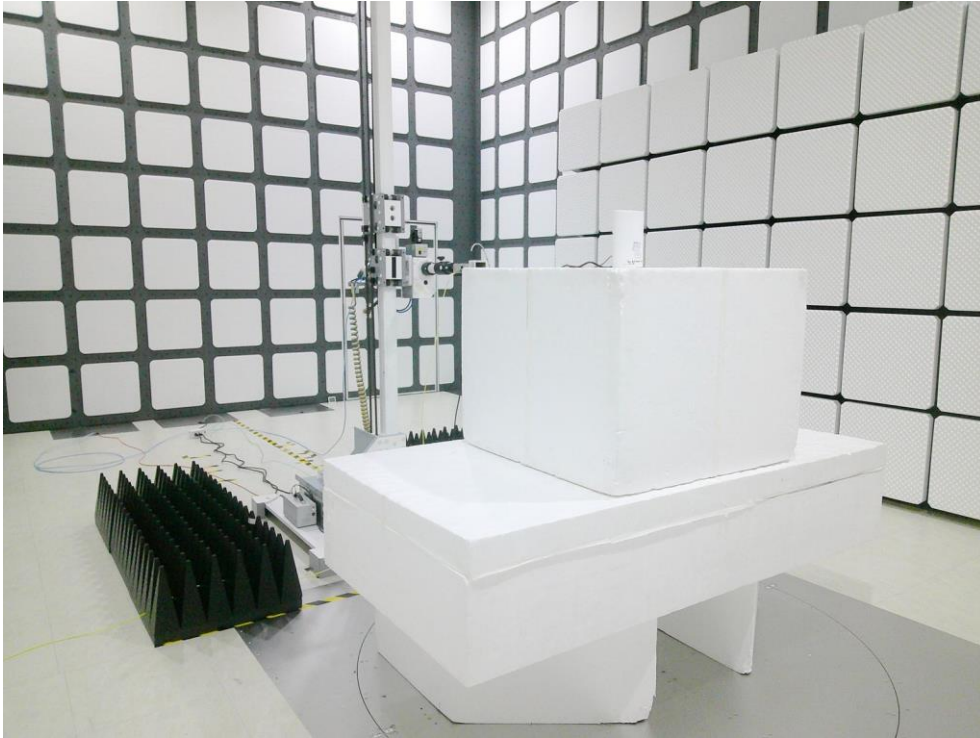
Description: Radiated Emission Test Setup for 9kHz~30MHz
