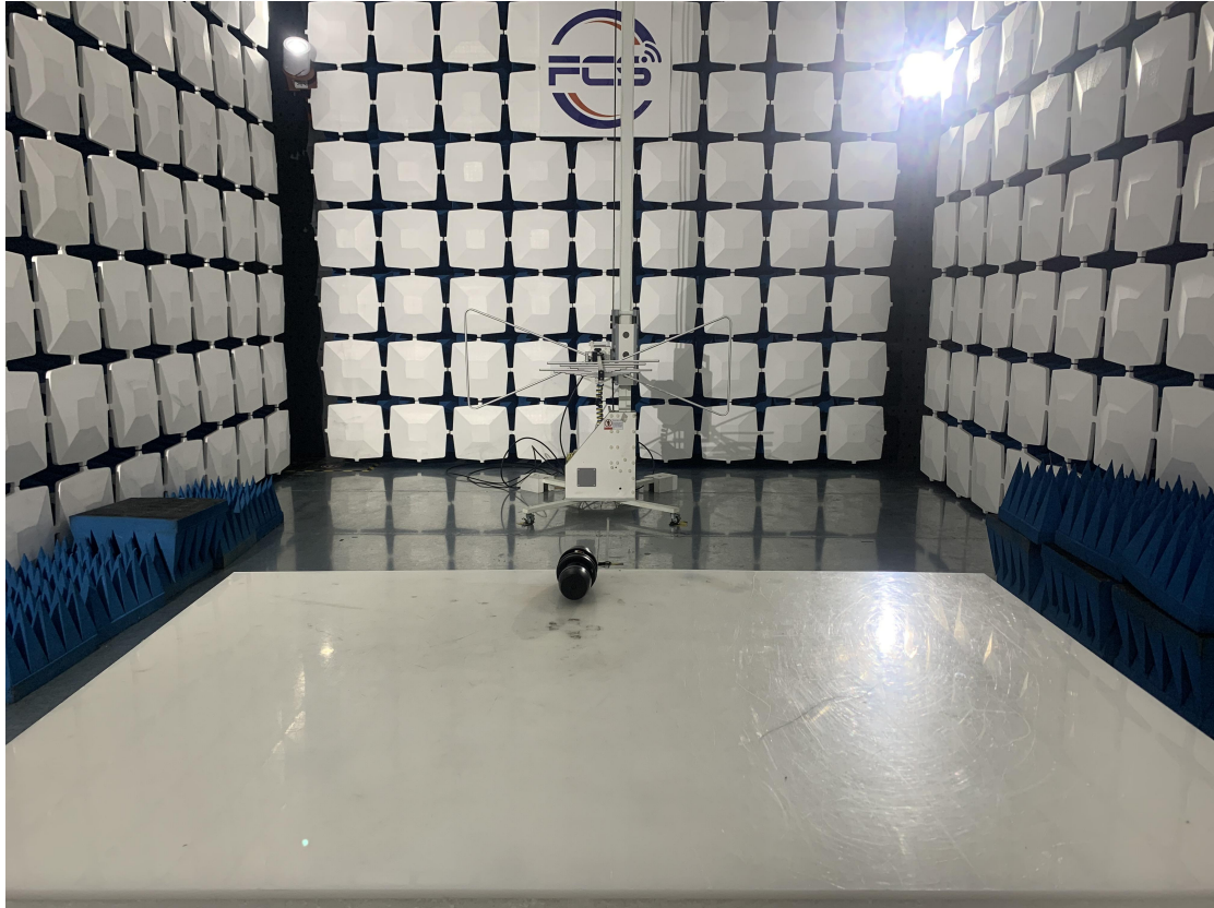
Above 1GHz for radiated emission test setup
