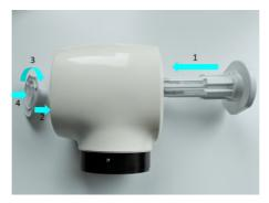
Figure 14 Sterile Interface insertion order
