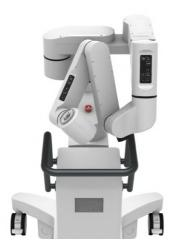
Figure 39 Example of compact boom configuration
