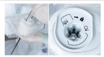
Figure 34 Emergency Release Tool and Sterile Interface
