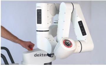
Figure 7 Release the emergency stop button clockwise
