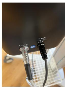
Figure 46 Example of a cable wrongly plugged
