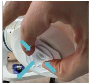
Figure 38 How to pull the Sterile Interface Lock away (Step 1 on the image above)
