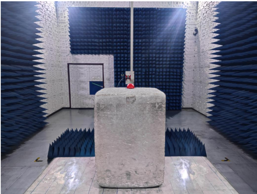
RADIATED EMISSION TEST SETUP ABOVE 1GHz
