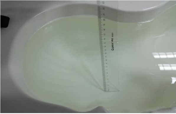
The Head Liquid of 1900MHz (15.5cm)
