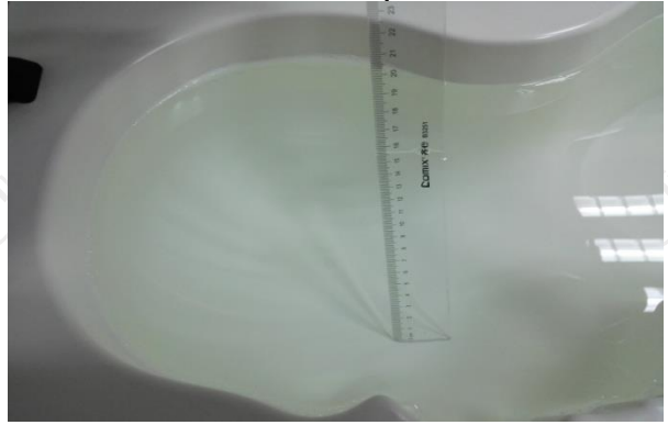
The Head Liquid of 2450MHz (15.6cm)
