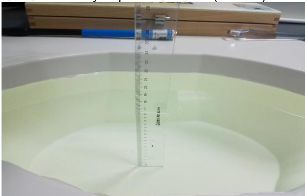
The Body Liquid of 1900MHz (16.4 cm)
