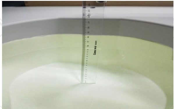
The Body Liquid of 1800MHz (15.2 cm)
