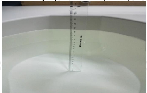
The Body Liquid of 2450MHz (15.3cm)
