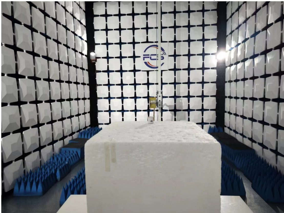
Above 1GHz for radiated emission test setup
