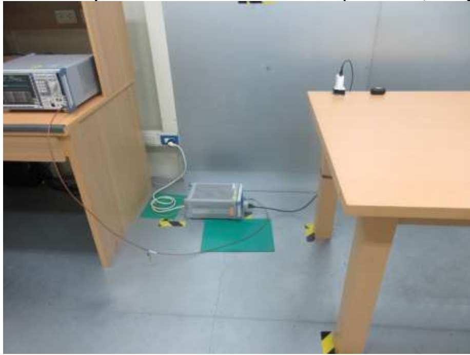
Photograph 14: Test Setup for Mains Conducted Emissions (Back View, Charge Mode)
