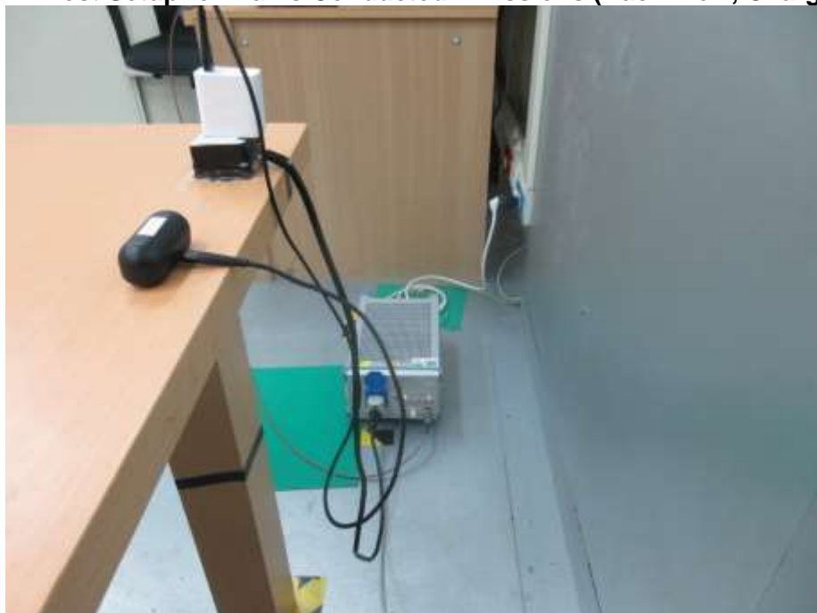
Photograph 14: Test Setup for Mains Conducted Emissions (Back View, Charge Mode)
