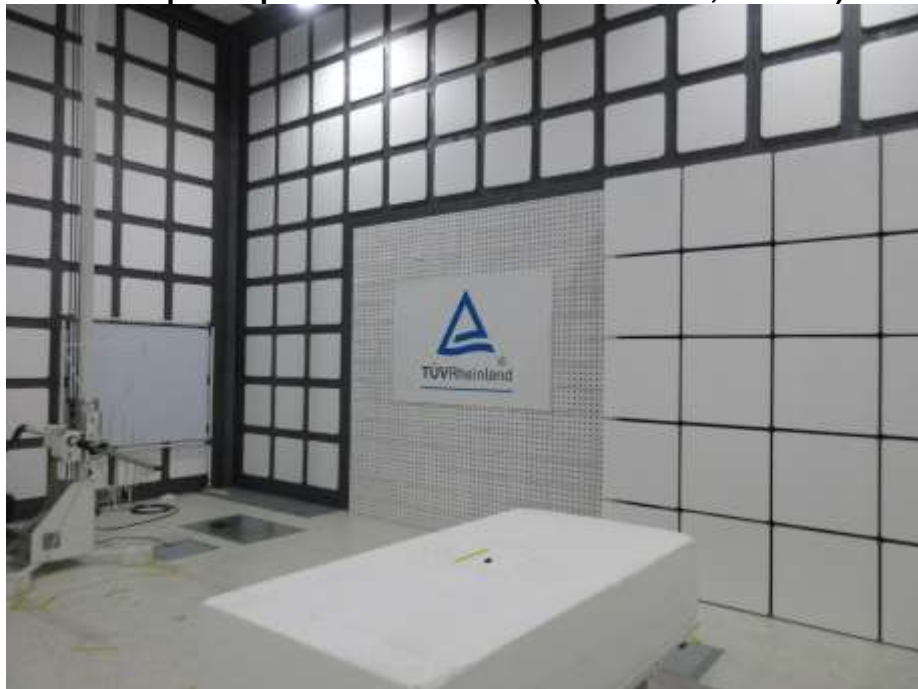
Photograph 4: Test Setup for Spurious Emissions (Back View 2, Left Ear)
