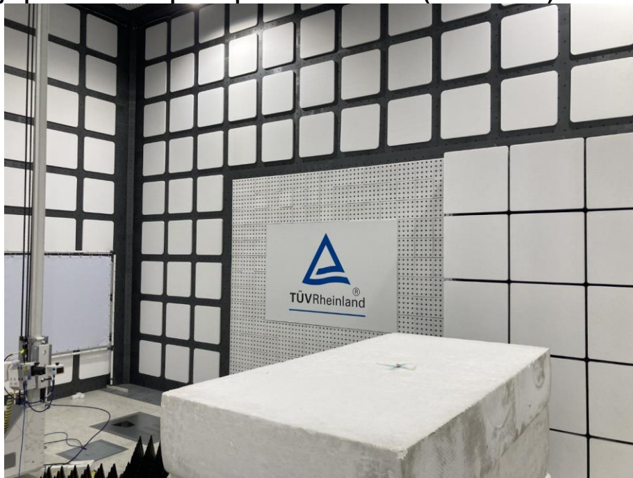
Photograph 6: Test Setup for Spurious Emissions (Back View 4)
