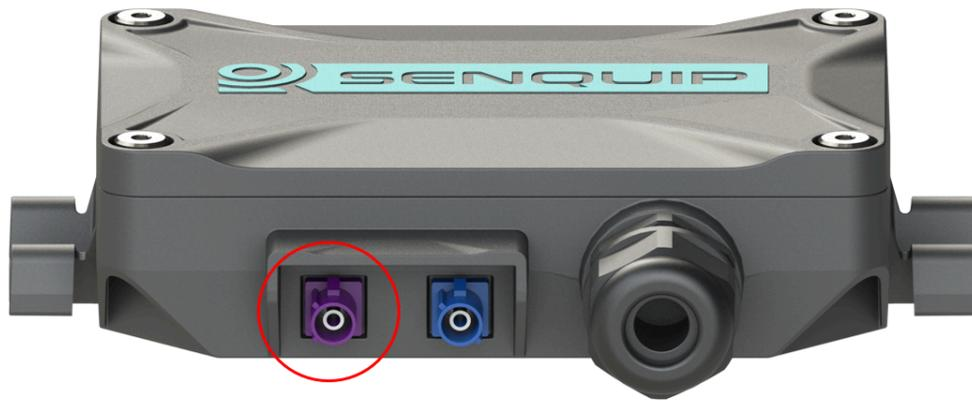
Figure 8.1. FAKRA-D 4G LTE antenna connector
