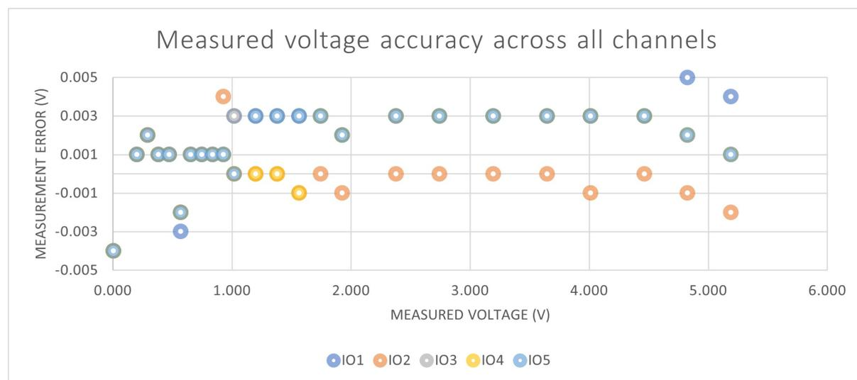
Figure 6.7. Voltage accuracy across all IO channels
