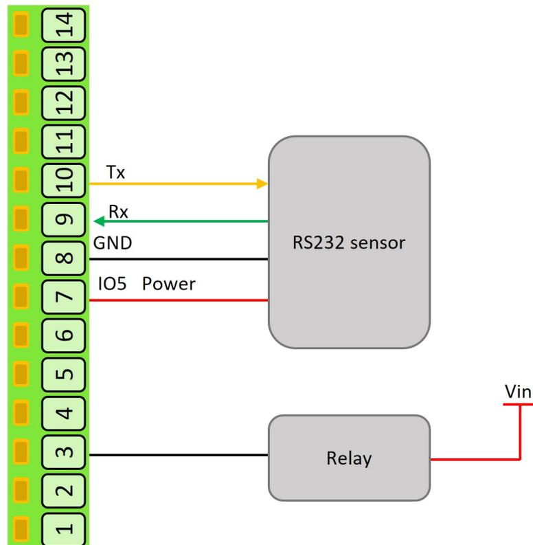
Figure 6.2. Powering external devices on an IO
