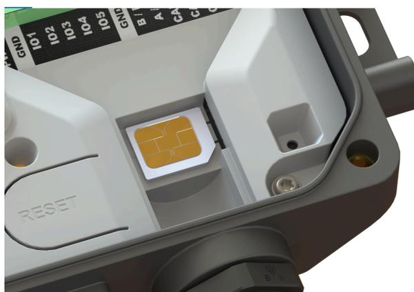
Figure 12.2. Remove the SIM card before opening.
