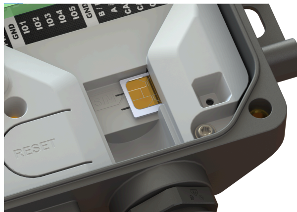
Figure 2.12. Insert SIM to the right
