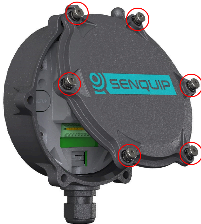
Figure 2.7. Six cover screws
