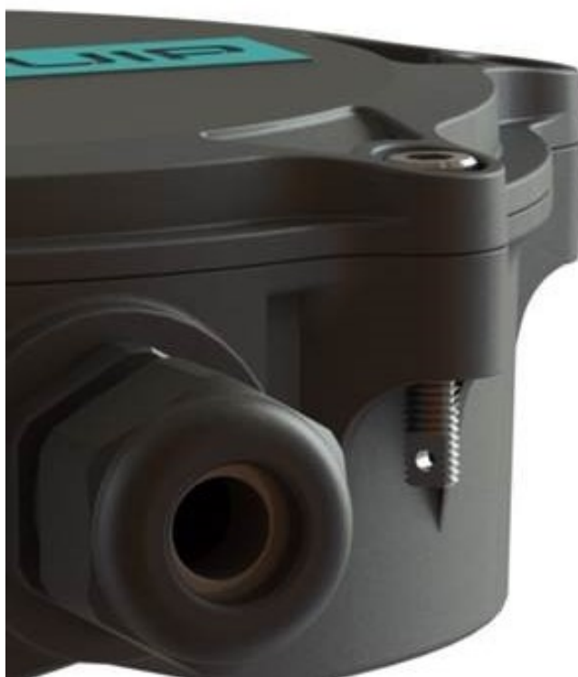
Figure 2.9. Tamper evident screw in place on an ORB
