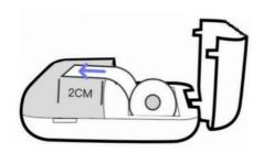
3. Cover the paper bin, the machine can automatically absorb paper after normal use.
