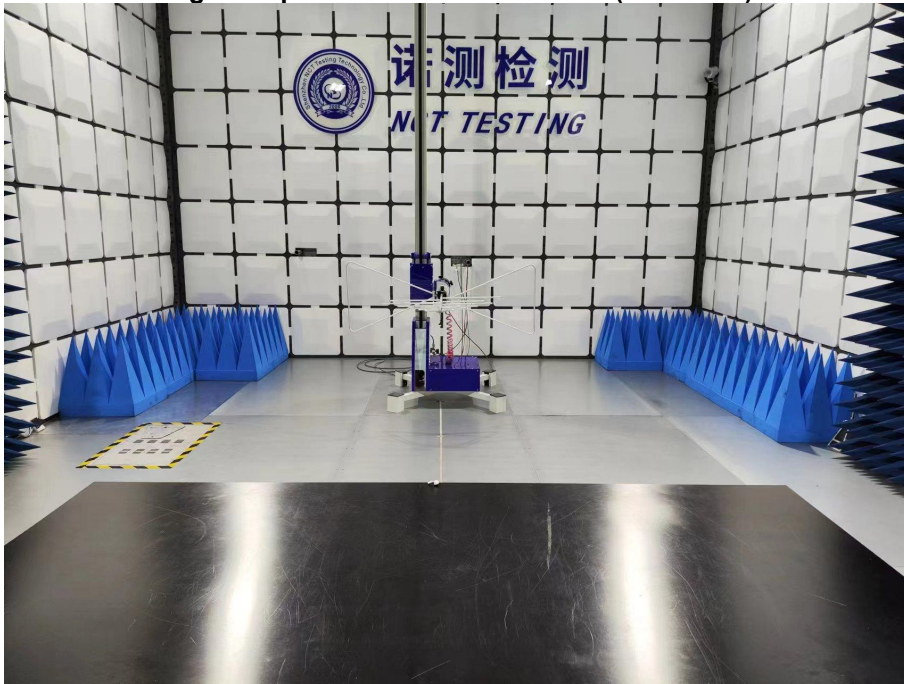
Right Earphone Radiated Emission (Below 1G)
