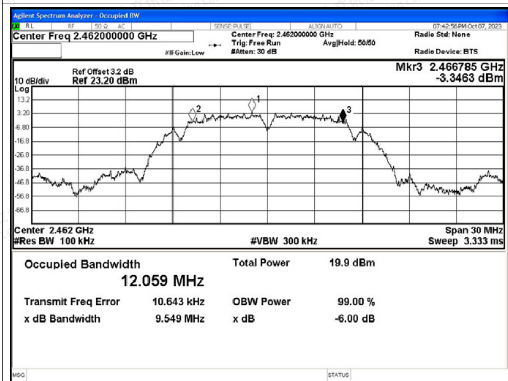
-6dB Bandwidth NVNT g 2412MHz Ant1
