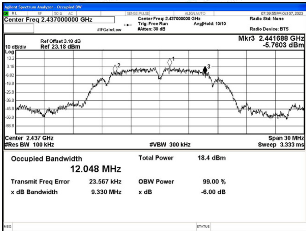
-6dB Bandwidth NVNT b 2437MHz Ant1
