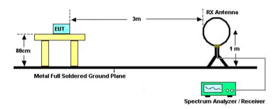
(B) Radiated Emission Test-Up Frequency 30MHz~1GHz
