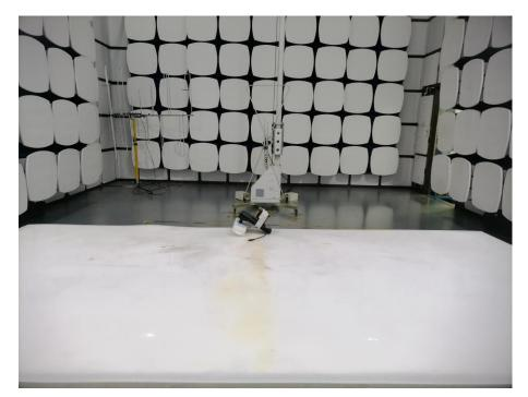
1.1. Photo of Radiated Emission test
