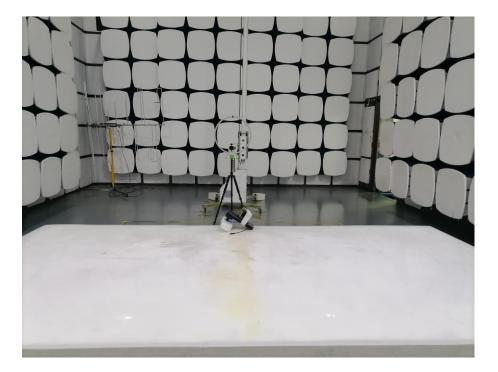
1.2. Photo of Conducted Emission test
