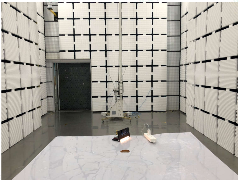
Radiated Emission below 1GHz-AC adapter charge mode
