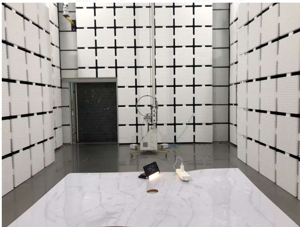
Radiated Emission below 30MHz-AC adapter charge mode
