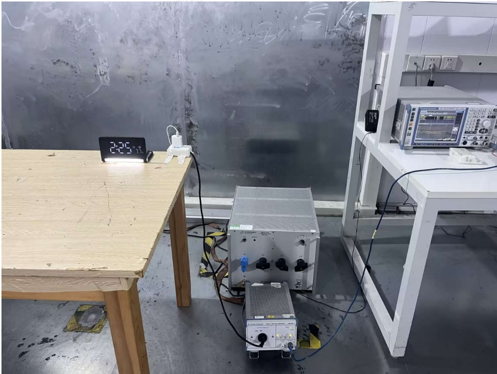
Conducted Emission-AC adapter charge mode
