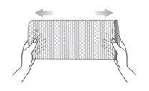
4 After cleaning, gently stretch the filter by holding it from top to bottom to prevent any changes in shape.
