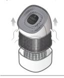
2 Lift the main unit to separate it from the water tank.
