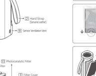
Secure the bottom of the filter cover onto the product and close it.
