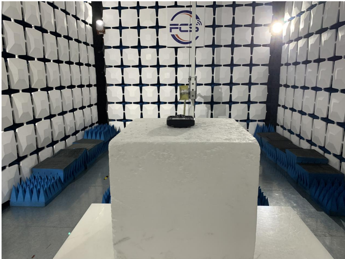
Above 1GHz for radiated emission test setup
