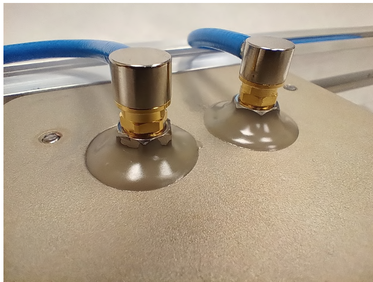
Figure 6: Covering the main unit RF connectors by LOCTITE EA 3425 epoxy adhesive
