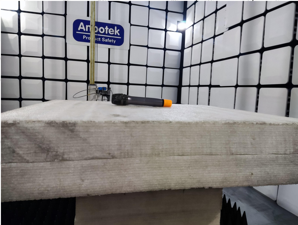
Photo of Radiation Emission Test (above 1GHz)
