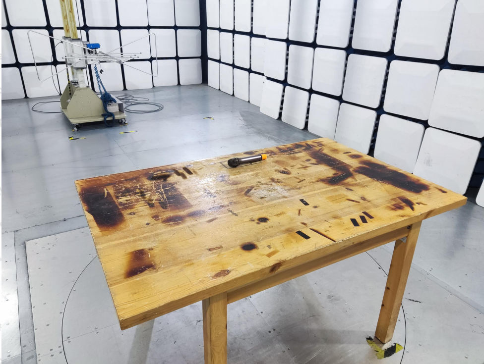
Photo of Radiation Emission Test (below 1GHz)
