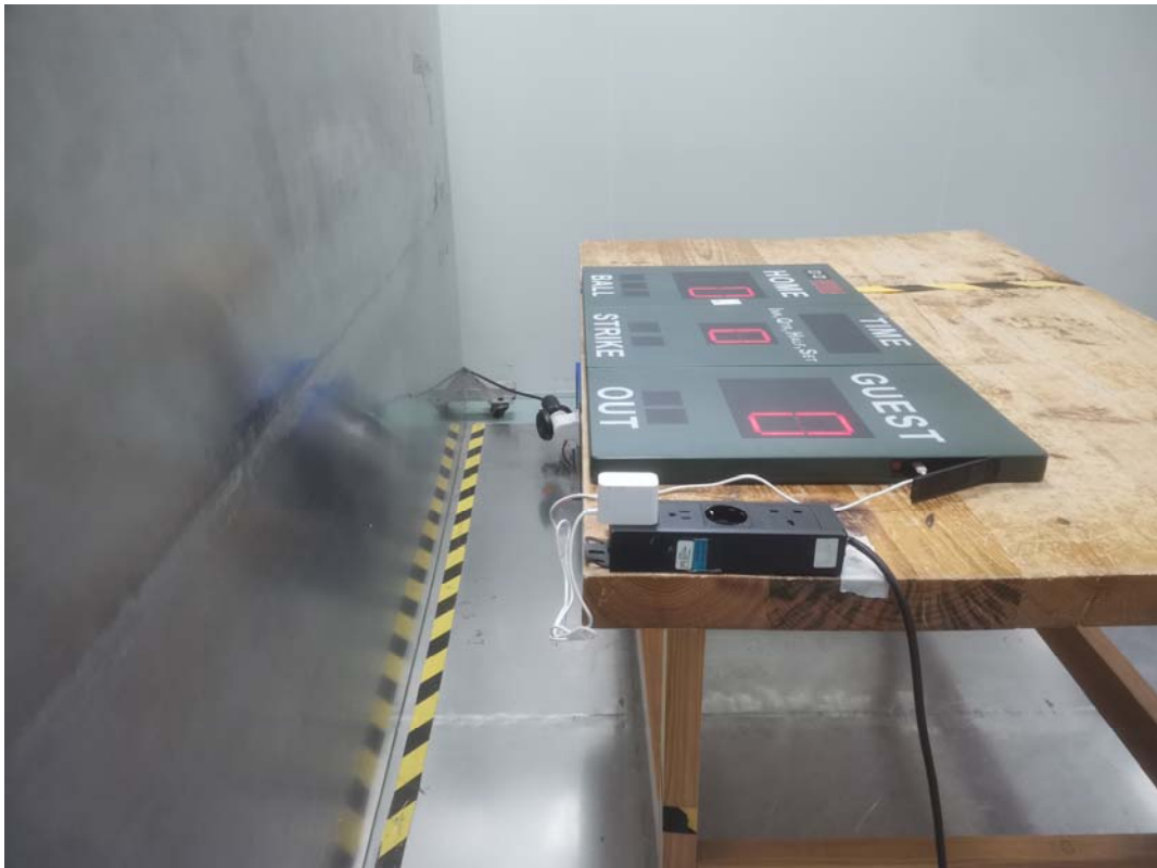
Conducted Emissions Side View-Adapter 1
