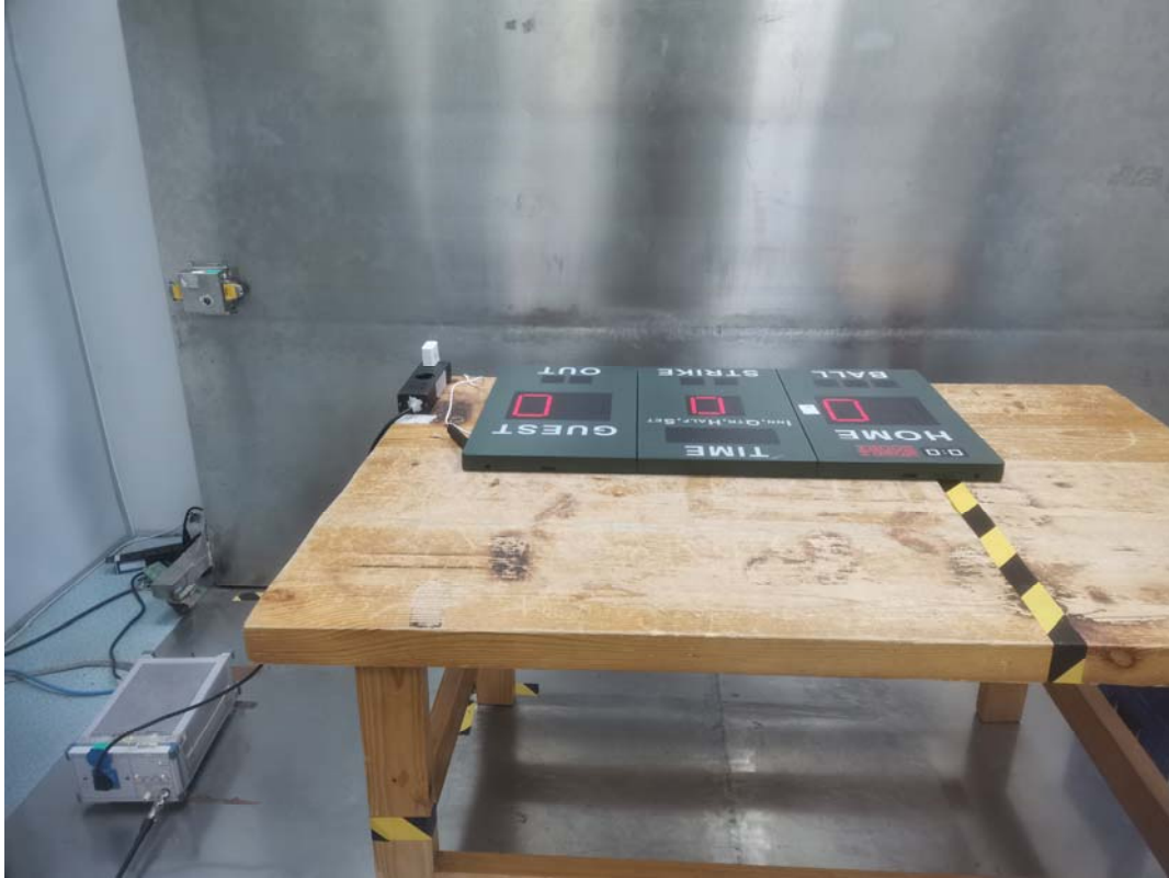
Conducted Emissions Side View-Adapter 1
