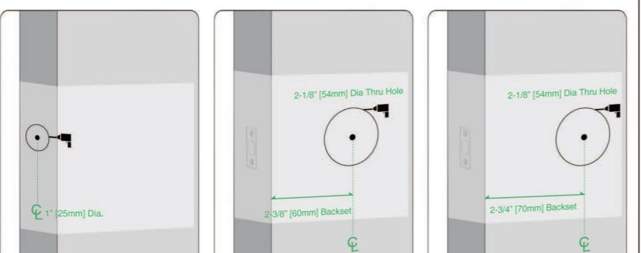
A: Use the Drill Measure Card or measure the middle of the door thickness to drill the center of the front door hole; drill the hole by 25mm (1 in) diameter.
